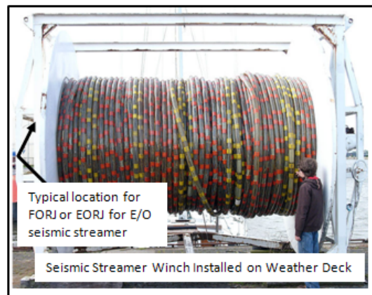
Figure 7 Locations for FORJ or EORJ Installations on Seismic Streamer Winch
